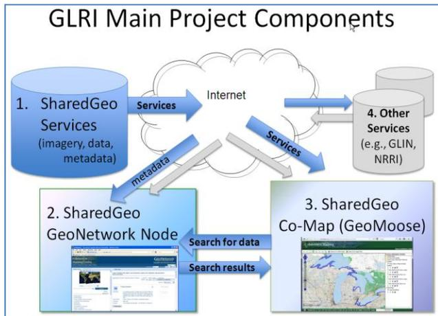
The raw imagery data, including radar, satellite and aerial photography are stored in a *Swift* storage. Then Image, Tile and Coverage services (WMS, WTS and WCS) are created and made available in the cloud. Metadata are also provided as part of these services.
